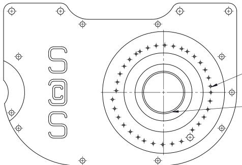
Use Centerdrill marks to drill holes at desired position
