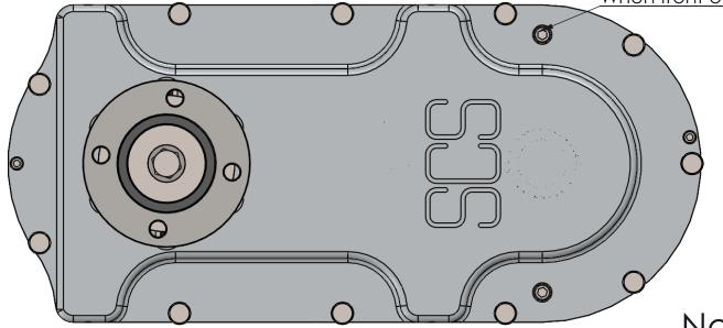
Note: Fill with 80-90 Synthetic Gear Lube Capacity: 1-1/4 Quarts
